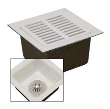
12" Square x 6" Deep Cast Iron Floor Sink with White Porcelain Coated Interior, Porcelain Cast iron Grate with White Porcelain Coating Plus Aluminum Dome Strainer.
